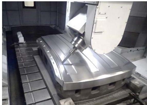
素材: FCD450 寸法: 1,850 x 1,300 x 615 mm
